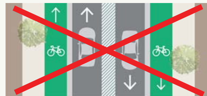
Protected bicycle lane on each side of the road and flush median strip in carriageway. No parking retained.
